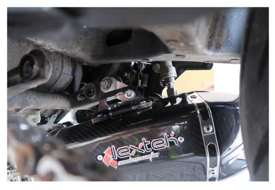
Loosely secure your new Lextek Silencer to the header using the mounting point (installed earlier).
