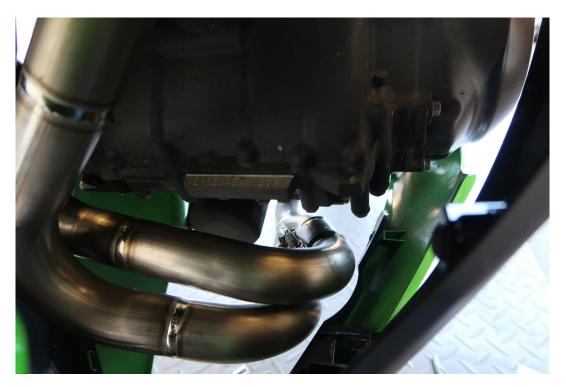
Tighten the header nuts to 20Nm torque setting and all clamps to 12Nm torque.
