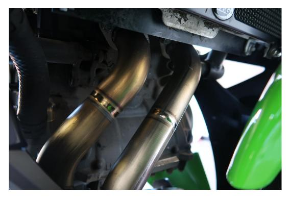
Add the middle section to the down pipes and secure with the springs provided.
